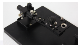
Magnetic holder to fix mouse body
