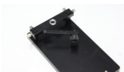
Slit to fix ring on the mouse skull
